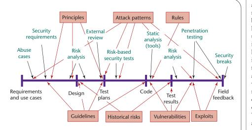
Figure 1. The software development life cycle. Mapping software security knowledge catalogs to various software artifacts and software security best practices shows us how various knowledge catalogs can be applied throughout the SDLC.
